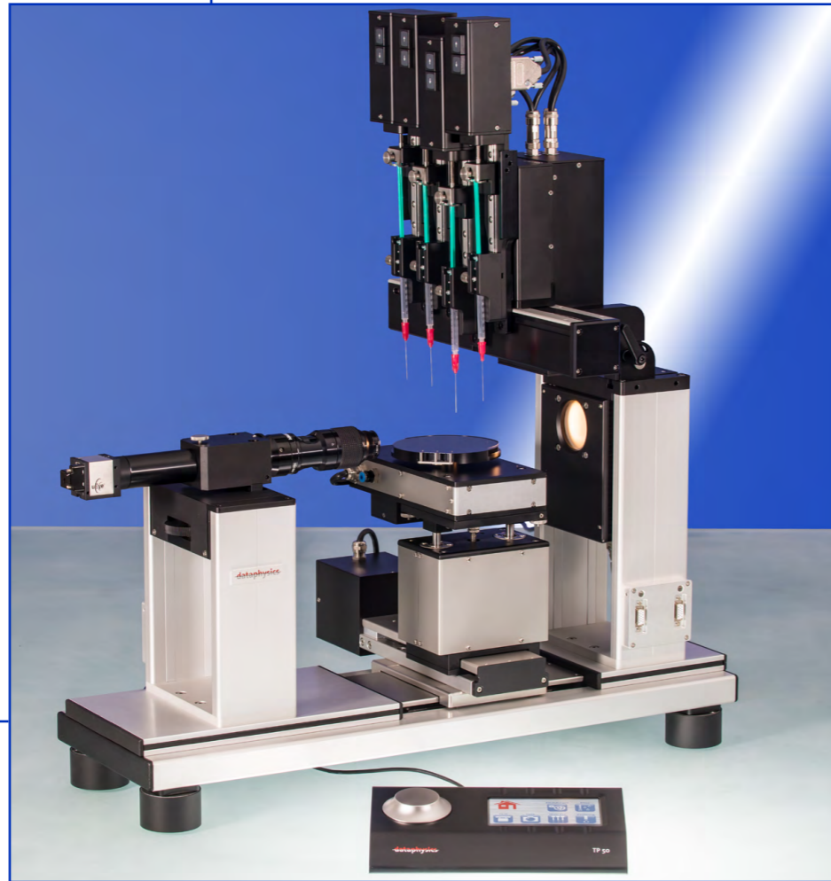
Automatic wafermapping with an OCA 50Pro with ETTr/Vac and DDE/4 with 4 ESR-D
